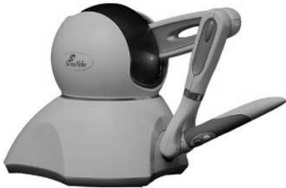
Figure 2. Three degree-of-freedom PHANToM Omni haptic device.
