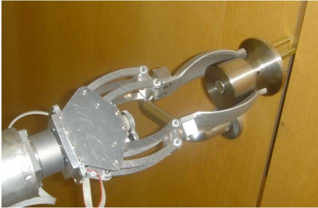
Figure 16. The new gripper when opening a knob handle door
