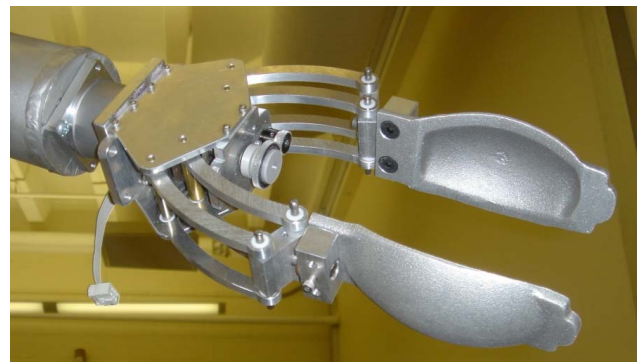
Figure 11. The new gripper and the actuation mechanism
