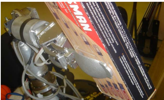
Figure 18. The new gripper when handling large objects
