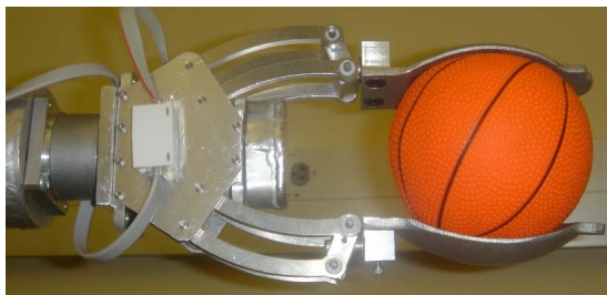
Figure 13. The new gripper when holding a spherical object
