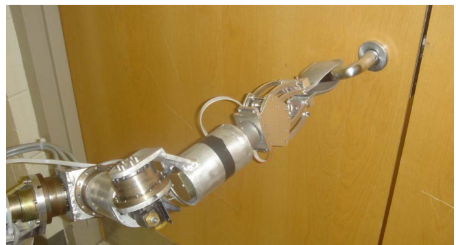
Figure 15. The new gripper when opening a lever-handle door
