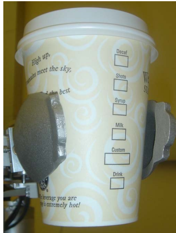
Figure 14. The new gripper when holding a tapered cup
