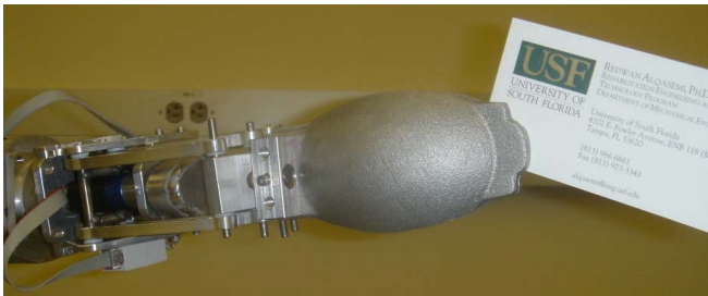
Figure 17. The new gripper when handling small objects
