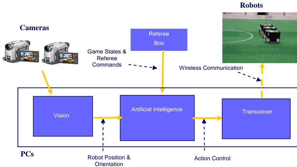
**Figure 3. RoboCup Small-Size league block diagram. Visual input from cameras mounted on top of the field are processed by the Vision module to provide the AI module with robot positions and orientations. The AI module sends action command to the robots via a transceiver.**
