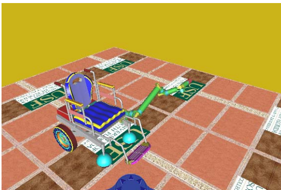
Figure 13: Destination pose when W_d = [1, 1, 1, 1, 1, 1, 1, 1, 100]
