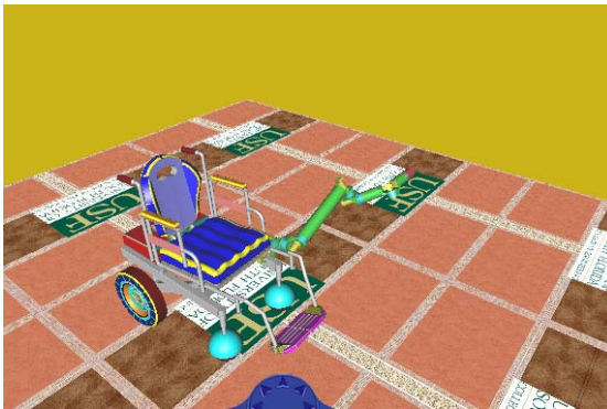
Figure 13: Destination pose when W_d = [1, 1, 1, 1, 1, 1, 1, 1, 100]
