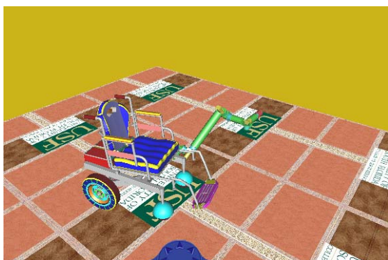
Figure 9: Destination pose when W_d = [1, 1, 1, 1, 1, 1, 1, 1, 1]
