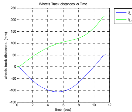
Figure 19: Wheels' motion when Wd = [1, 1, 1, 1, 1, 1, 1, 1, 1]
